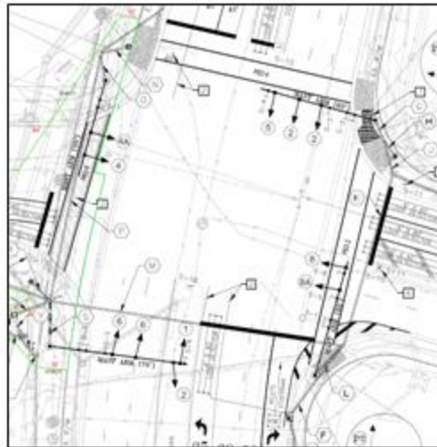
Poles in quadrants with utility conflicts
