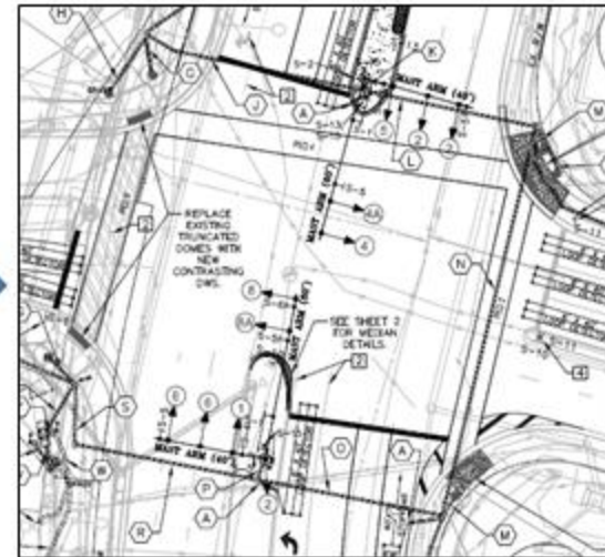
Poles in median with no utility conflicts
